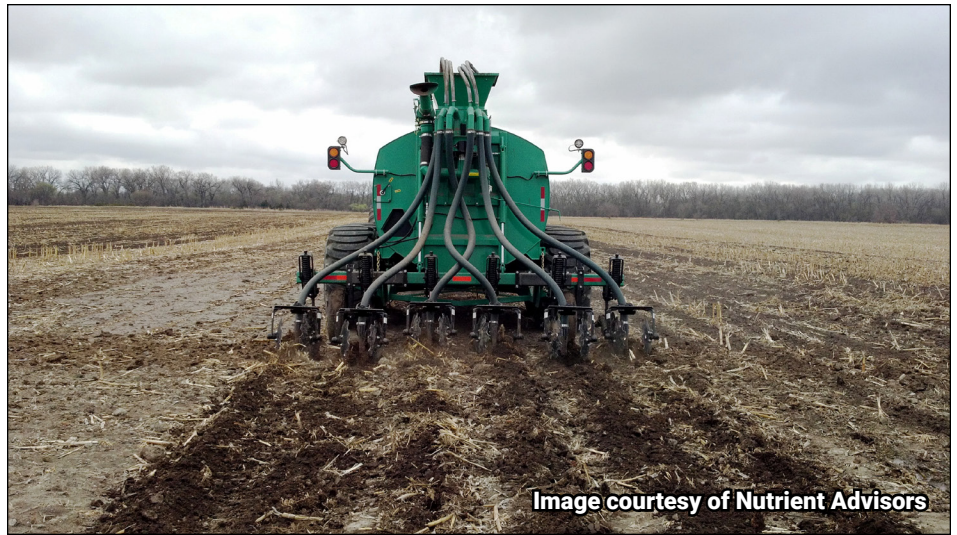
Slurry (manure in liquid) being injected into the soil.
